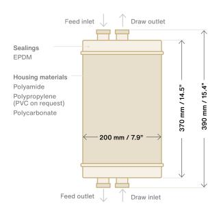
Weight, dry 4 kg (8.8 lbs) Weight, filled with liquid 7 kg (15.4 lbs)
