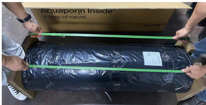
Figure 3: Unpacking the RO FS roll: lift the roll from the carton box using the packing straps
