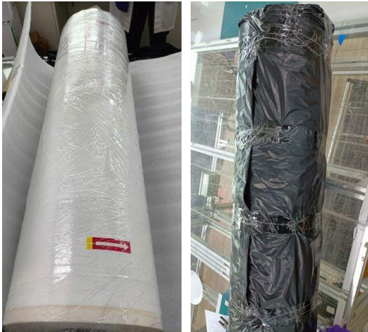
Figure 5: Repacking the RO FS roll: wrap the RO FS roll with stretch film wrap and replace the padded wrap around the roll (left); replace the black wrap around the roll (right).
